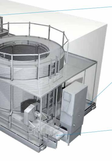
Fans located on dry side of evaporator Optimized air velocity through evaporator.
