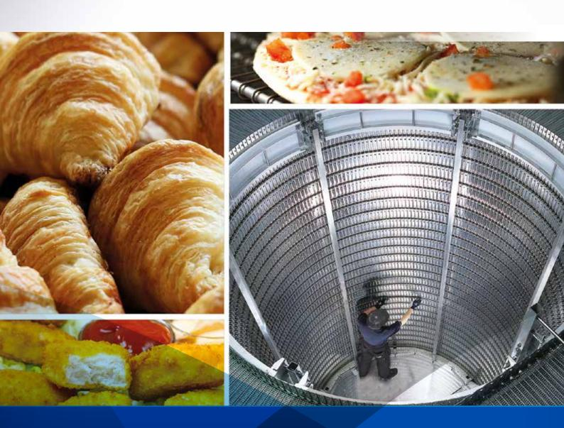
Highly modular and flexible self-stacking spiral freezer
