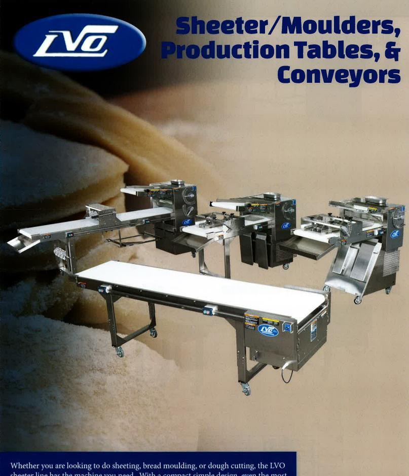
Whether you are looking to do sheeting, bread moulding, or dough cutting, the LVO sheeter line has the machine you need. With a compact simple design, even the most inexperienced employees can sheet dough in seconds. With different attachments available for moulding or cutting, making bread loaves, donuts, croissants, turnovers, and other pastries becomes automatic and uniform.
