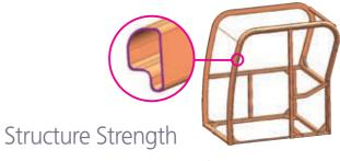
The 9 series cabin structure has been fitted with stronger but slimmer tubing for more safety and improved visibility. Low-stress, high strength steel is integrally welded to form a stronger, more durable upper and lower frame. Structural integrity was tested by way of FEM (Finite Elements Method) analysis and long-term durability tests.
