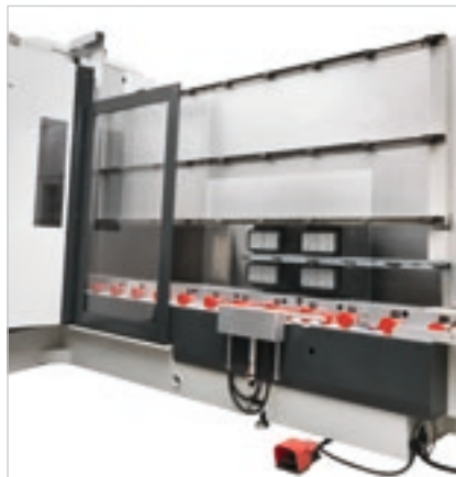
Equipped with idle rollers (that can be motorised if required) on the machine infeed.
