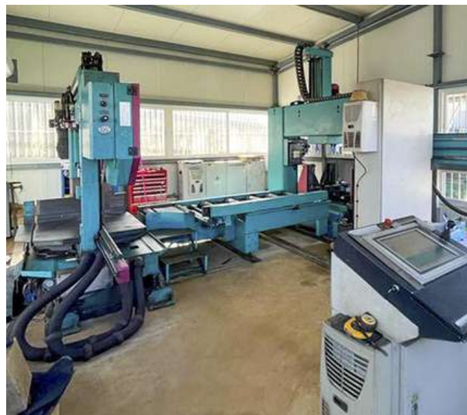
BEAM LINES & COPING ROBOTS
