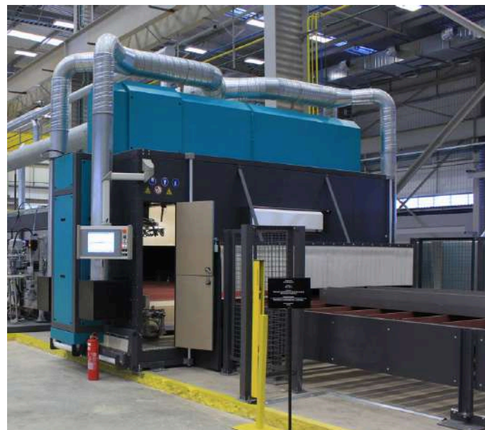
SHOT BLASTING & PAINTING SYSTEMS
