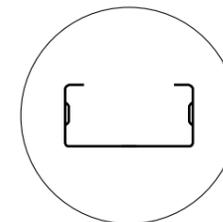
Web width range from 89mm to 150mm (3.5" - 6"). Gauge range from 0.95 to 2.0mm (20 - 14 gauge).
