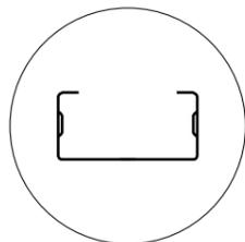
Gauge range from 1.2mm to 2.3mm (18 - 13 gauge), C profile range from 250mm - 305mm (10" - 12")
