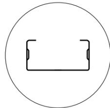
Web width range from 50mm to 300mm (2" -12"). Gauge range from 0.60 to 2.0mm (24-14 gauge).
