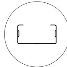
Web width range from 92mm to 305mm (3.625"-12") with up to 4 profiles. Gauge range from 0.85mm to 2.0 mm (20-14 gauge).
