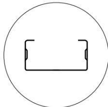
Web width range from 40mm to 63mm (1.625"-2.5"). Gauge range from 0.55mm to 1.2mm (24 - 18 gauge).
