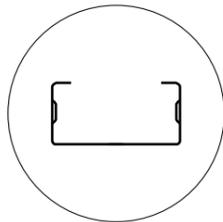
Web width range from 89mm to 203mm (3.5"-8") with up to 4 profiles. Gauge range from 0.70mm to 1.6 mm (22-16 gauge).
