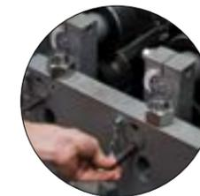
A simple and intuitive gauging system allows for quick change of gauges between 1.2 - 3.2mm (18 - 11 gauge) steel.
