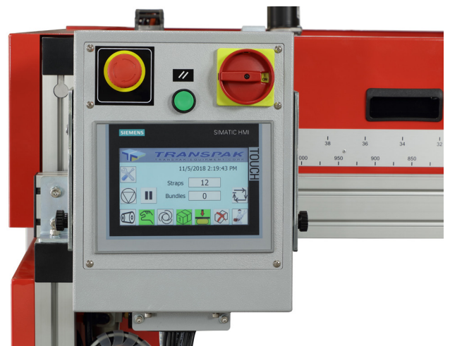
Siemens PLC and HMI
