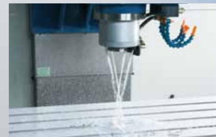
Coolants Jets Around Spindle Improved cooling efficiency on workpiece. (ISO 40 standard, ISO 50 optional)
