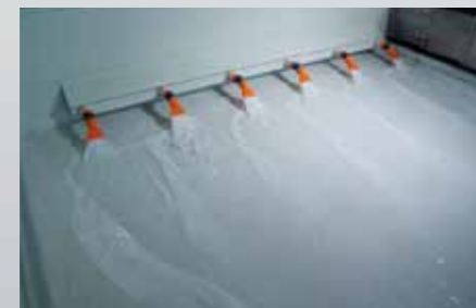
Cools Flushing Nozzles Coolant flushing nozzles on rear inner wall of guard prevent jam of chips during operation.
