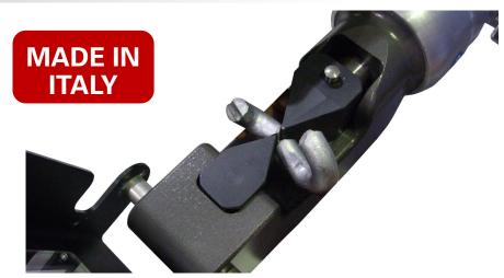
The TC26M electric hydraulic chain cutter is a precision engineered hydraulic tool that can be used to cut through 26mm maximum high tensile chain. The TC26M cutting head is hydraulically driven by a reliable double insulated motor which drives a precision designed radial hydraulic pump that produces up to 31 Tons of pressure.
