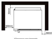
\*Clearance requirements \*Drain line must be vented
