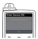
10. Pick up the pump. Enter the meter serial number (SN) shown on the meter into the pump screen. Use the up and down buttons to select the characters, then press the right button to move to the next character. Keep pressing up to get to the alphabet. Press down to go in reverse (starting with "Z"). Press the Select button after entering the last SN character. Select OK on your pump.
