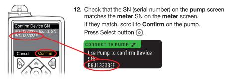
When the pump links to the meter, the SN on the **meter** screen will change to a different serial number. This number is the **pump** SN.
