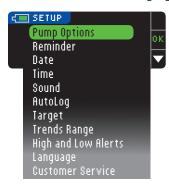
The current settings in the meter for the Reminder, Date, Time, Sound and AutoLog can be viewed by scrolling through the Setup Menu items. To view the settings of the other items, or to make any changes to any of the items, you can select the item using the ▲ and ▼ keys and pressing OK.
