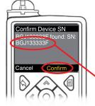
**13.** Check that the Device SN (serial number) on the **pump** screen matches the **meter** SN on the **meter** screen.
