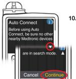
**10.** Read the pump screen. Be sure other nearby Medtronic devices are NOT in search mode. Use the down arrow to scroll to the next page. Use arrow buttons to scroll to **Continue**. Press Select button .
