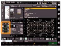
Touching the buttons to adjust the EDM parameters
