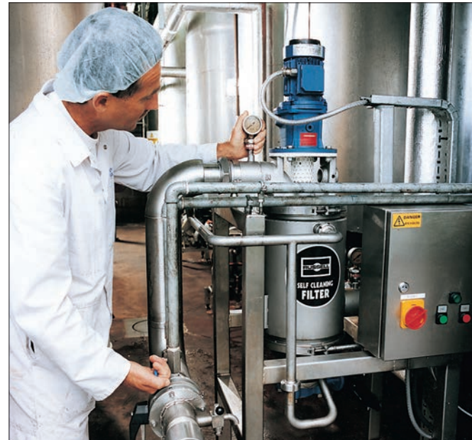
Self-Cleaning Russell Eco Filters® aid quality control procedures for filtering liquid chocolate at Walls Ice Cream.
