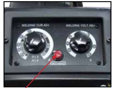
(10) Press and hold the inch wire button to feed the wire down the torch cable through to the torch head.
