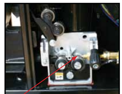
(7) Feed wire over the drive roller into the outlet guide tube, Push the wire through approx 150mm.
