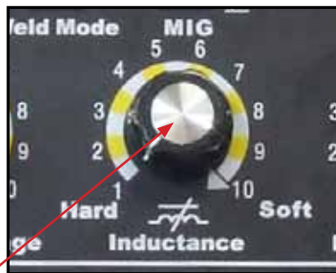
(15) Set the inductance control on the front panel of the power source to get the desired arc characteristic. Less inductance for a TIGHT hard arc and more for a soft wider arc.
