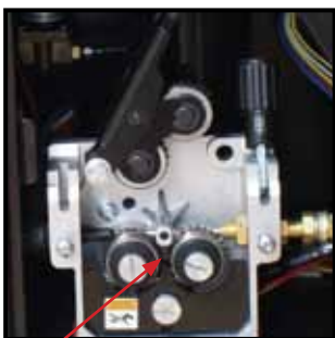
(8) Fit the correct type and size of drive rollers. V Groove for Hard Wires. Knurled for Flux Cored. U Groove for Aluminium.
