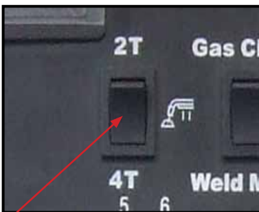
(1) Select 4T trigger function using the trigger control function switch located on the front panel of the power source.
