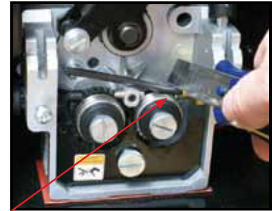
(15) Cut the extended PA liner with a sharp Stanley knife just in front of the drive roller
