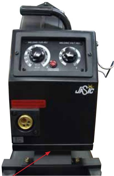
(4) Place the wire feeder by locating the mounting hole on the wire feeder base over the locating pin on the wire feeder mounting bracket.
