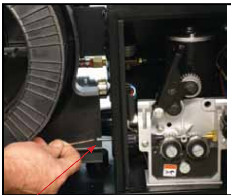
(4) Snip the wire carefully, be sure to hold the wire to prevent the spool uncoiling. Carefully feed the wire into the inlet guide tube of the wire feed unit.
