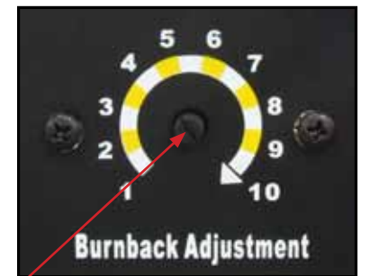
(16) Adjust the burn back control to prevent the wire sticking in the weld pool. Burn back control is located on the rear panel of the power source
