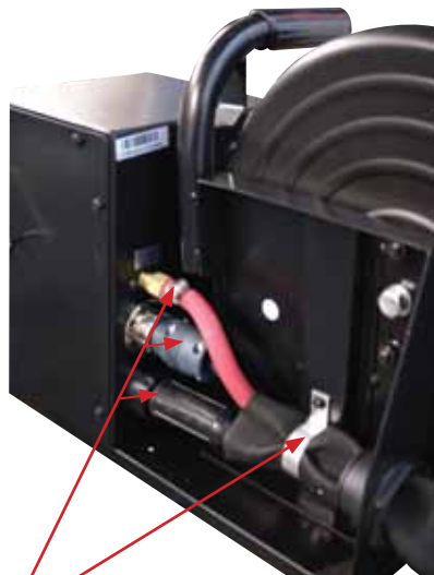
(5) Connect the control cable assembly and fasten firmly in place with the cable retaining bracket.
