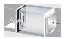
Cold Jet's patented feeder technology creates shaved dry ice on demand, regardless of input.
