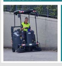
The ASC G5 has a climbing capacity of up to 25%, making it ideal for car parks and other sites with ramps and high inclines.
