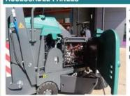
The G5 is designed with easily assessable components, with all panels able to be removed in seconds.
