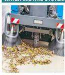
Fitted with a water spraying system, the ASC G5 effectively eliminates airborne dust.
