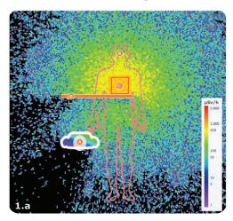
In order to test the efficiency of a shielding curtain, the scattered radiation distribution was simulated using the Monte Carlo method for the new radiation protective shield both with and without a curtain. See fig. 1.a and 1.b
