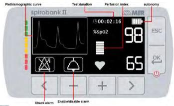
To end an oximetry test press **ESC** key.
