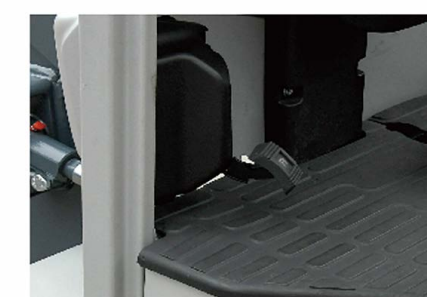
New pedal parking system, ergonomic design, very convenient
