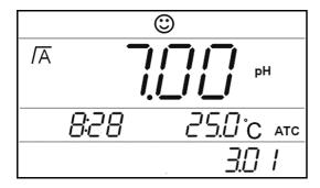
icon, the instrument will block the measurement value, the value could be read. In left chart, the date is 1st March, time is 8 o'clock 28, the sample temperature is 25.0°C, automatic temperature compensation (ATC), auto
