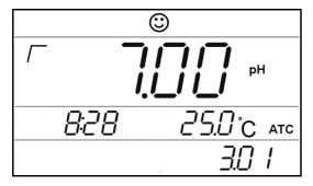
"\scale" "icon if the measurement is stable, the measurement value could be read. In left chart, the date is 1st March, time is 8 o'clock 28, the sample temperature is 25.0°C, automatic temperature compensation (ATC), auto ending
