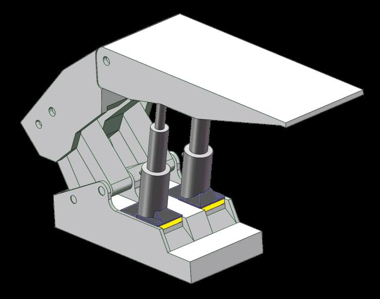
To ensure the perfect fit for your longwall, we take measurements of your leg pockets and model a specific foam filler to fill the void.
