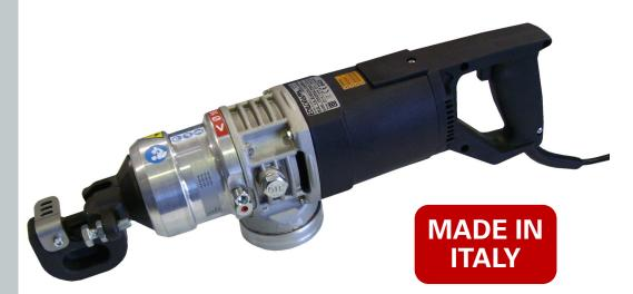
Designed for cutting 16mm high tensile material Silvercut 16 electric hydraulic rebar cutter features a powerful 230V motor which drives the precision radial hydraulic pump to produce 13 Tons of cutting force.
