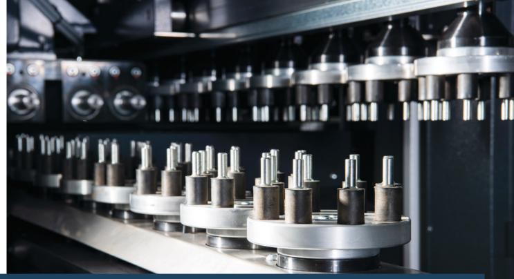
The EdgeBreaker® 5000 MAX removes slag caused by plasma and oxyfuel cutting.
