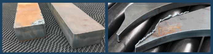
Flame cut parts before and after processing with the EdgeBreaker® 5000 MAX.
