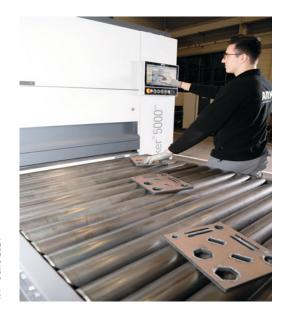
■ With the EdgeBreaker® touchscreen HMI you can easily save processing parameters in the tool storage. These stored parameters can be called upon at anytime.
