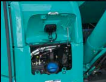
Ground level DEF tank
