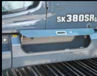
Ground level storage compartment access
