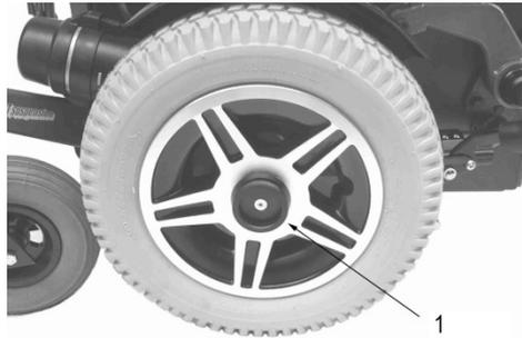
To ENGAGE, simply turn Black Knob (Drive clutch) in either direction until you here a “click”. Turn chair on and SET AT SLOWEST SPEED and then SLOWLY move joystick forward until drive clutch self engages. When clutch is engaged fully, the outer face of the Drive clutch will be flush with the retainer washer.
