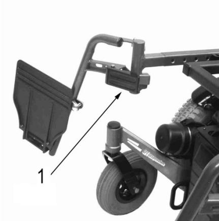
When refitting footrest to wheelchair ensure that it is located on both locating pins. Damage may result if only one pin is used. Once the legrest is on the locating pins and with foot plates up, swing legrest towards centre of chair firmly so latch will click into position.
