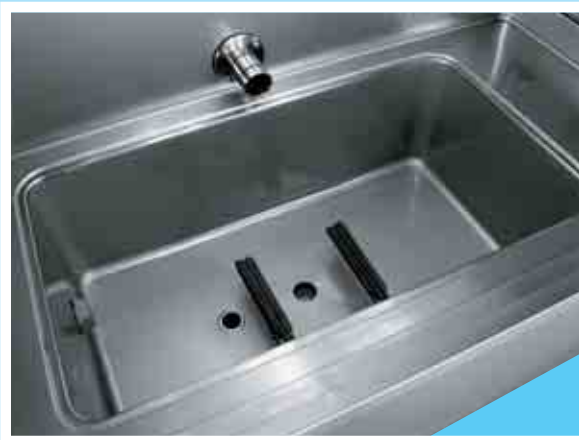
Pressed tanks in the pre-wash, wash and rinse zones, sloped towards drain to prevent dirt build up.
