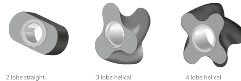
The rotor geometry and material are selected for the characteristics of the pumped media. Geometries are available for products which are viscous, abrasive or contain solids. Materials tailored to the media characteristics increase the durability of the rotors and extend service life.
