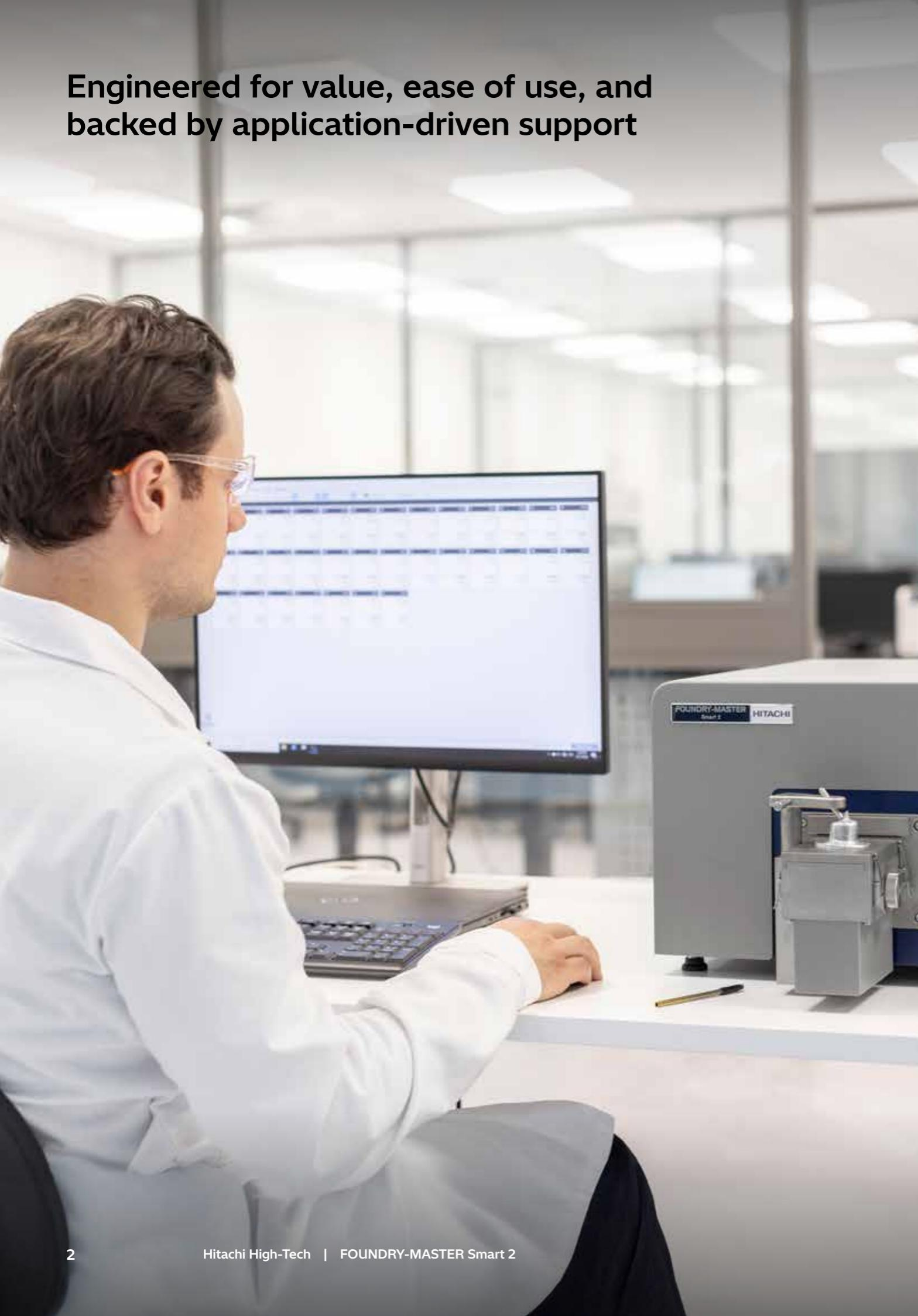
The FOUNDRY-MASTER Smart 2 delivers lab-grade precision in a compact, durable format built for the realities of industrial QA/QC. At its core is Hitachi High-Tech's precision engine: a pairing of CMOS sensor and ultra-stable spark source that ensures consistent, repeatable results for critical elements like carbon and nitrogen.
