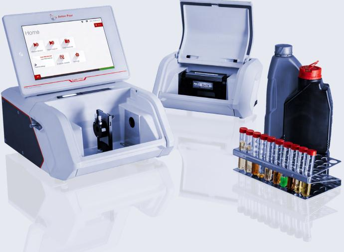
Lyza 7000 is a benchtop FTIR spectrometer for oil condition monitoring, compliant with the most important ASTM standards. Perform compliant analyses at the push of a button with pre-installed methods or configure your own individual methods based on your requirements.
