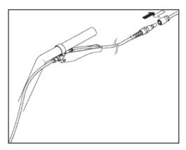
5. In the same way, you must connect the vacuum hose to the machine and to the accessory handle.
