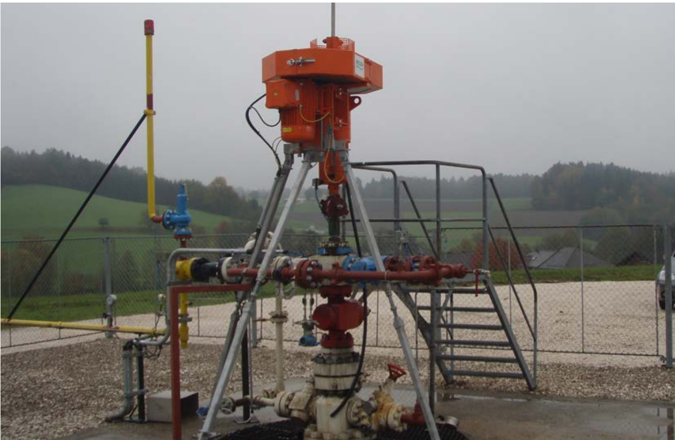
NETZSCH PCP System dewatering of a gas well in Austria
