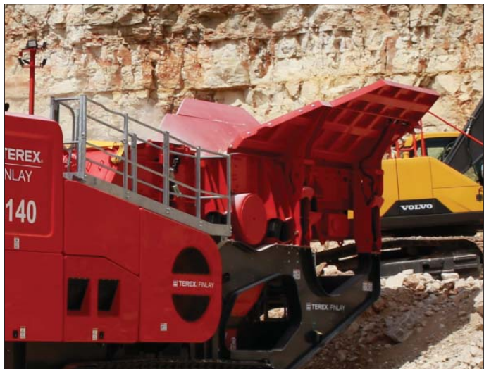
Hopper and Feeder
