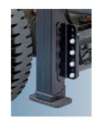
The photo shows outrigger beam non-extension type.
