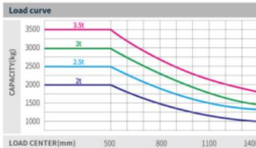
**Note:** The vertical axis stands for load capacity and the horizontal axis stands for load center which is calculated from the front surface of the forks to the gravity of the standard load. the standard load means a cubic with 1000mm edge length. When mast is tilted forward, using non-standard forks or loading large goods, the load capacity will be reduced. The load capacity of standard mast at different load center can be known from this load chart.
