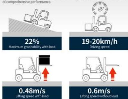
Note: the data displayed are all based on the model CPD30-GB2U-H, and data for other trucks are shown in the table of technical parameters.
