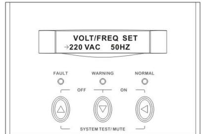
C. Use Up or Down-key to adjust the output voltage (if 220V configuration, 220V, 230V, and 240V is selectable; if 110V configuration, 100, 110V, 115V, and 120V is selectable). Press Enter-key to confirm voltage and then the cursor will move to frequency selection. The output frequency (50Hz or 60Hz) can be adjusted by the same key operation.
