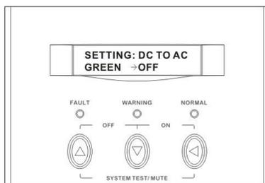
C. Use Up or Down-key to select the Green Power On/Off. Press Enter-key to confirm, and then the cursor will move to the time adjustment. The time period (15Sec., 30Sec., 45Sec., and 60Sec. is selectable) for next detecting can be adjusted by the same key operation.
