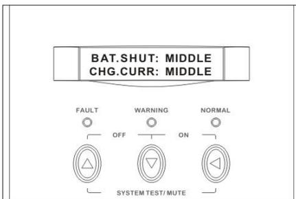
B. The cursor (→) will pop up to indicate the battery shutdown voltage.
