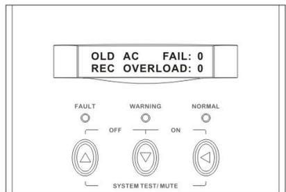
5. Input Voltage Range Setting - After inverter startup, press the Down-key to find the screen and then press Enter-key for setting.
