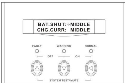
C. Use Up or Down-key to adjust the battery shutdown voltage (if 24V configuration, HIGH: 21V, MIDDLE: 20V, LOW: 19V is selectable).
