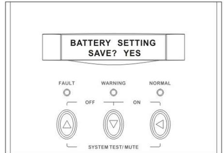
D. Once the correct battery charging current is selected, press Enter-key again to save the selection.
