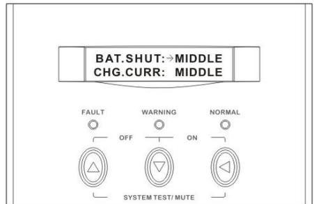
C. Use Up or Down-key to adjust the battery charging current (LOW: 100AH, MIDDLE: 300AH, HIGH: 600AH is selectable).
