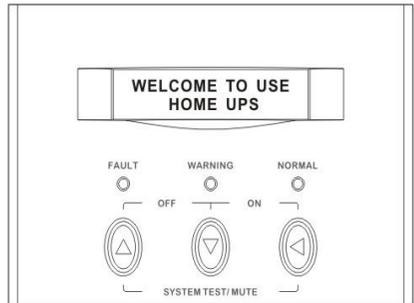
1. Once the AC source is connected, the LCD will light up immediately (8~10 seconds showing the greeting message) and revert to standby for inverter startup.
