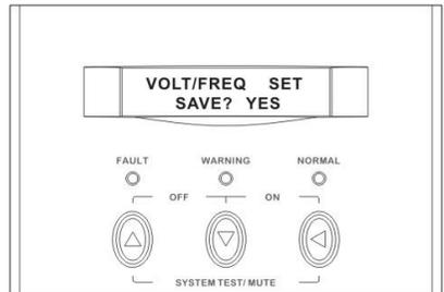
E. Turn off the unit and then restart it to enable the setting
