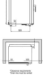
Heat Source: 500mm clearance from an external heat source is required in order to protect the oven control components and allow access to the service panel. For clearances under 500mm, it is mandatory for Stoddart heat shields to be fitted while still maintaining a minimum clearance of 300mm to provide access to the service compartment. Failure to adhere to minimum clearances may void the oven warranty or add service costs due to lack of access.
