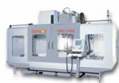
• VMC-2150 Vertical machine center 400MM ~ 3200MM X axis travel
