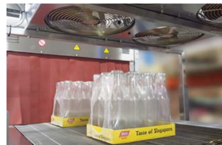
Cooling fans at outfeed
