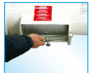
7 Inspection Hatch under inlet
