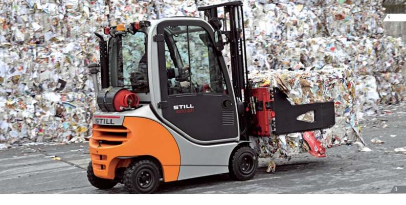
/ D + E Operation. The standard mini-lever and the optional Joystick 4Plus or fingertipp operation enable particularly precise and easy truck control.
