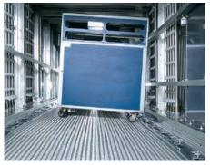
Unique belt design – Always level in the loading and unloading areas, the transport belt tilts to an angle during the washing process. This is to allow for a better flowing off of residual water from inside and outside the trolley, creating the necessary preconditions required for outstanding drying results.
