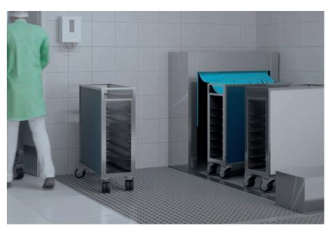
Optional clean zone – For optimal hygiene and process reliability the workspace can be separated into a soiled and a clean area.
