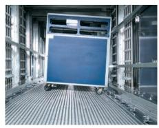
Clever drying technology – Once loaded into the washer, the transport tilts the trolley to facilitate residual water flowing off the trolley's internal and external surfaces for the best drying results.
