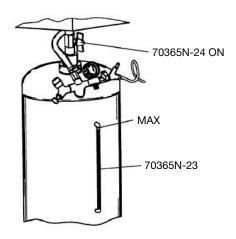
Phase 3: fill up the tank with the detergent.
