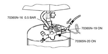
Phase 4: connect the compressed air, open slowly the cock (part 19) and make the regulation of the reducer (part 20) (the manometer (part 16) must point 0.5 bar.)
