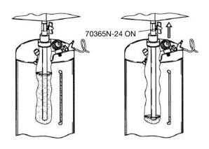
Phase 4: with the cock (part 24) open the pipe of the draught in the middle to allow the flow of about 20L of the detergent.
