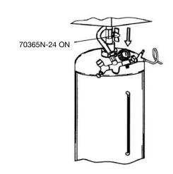
Phase 1: close the cocks (parts 24, 15, 19 and 20), close the reducer (part 20) and discharge the reservoir (open the valve (part 21)). In the discharge leave the valve open (part 21).
