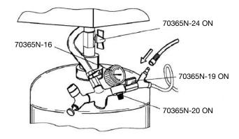
Phase 3: connect the compressed air, open the cocks (part 19 and 24) and make the regulation (part 20) gradually whilst paying attention to the movement of the detergent in the tank (a flux very strong can cause splashing and discharge).
