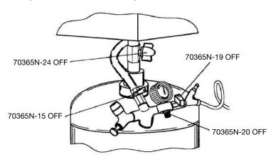
Phase 1: check that the cocks (parts 15, 24 and 19) and the reducer (part 20) are closed.
