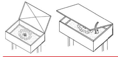
Phase 5: the flux of the air agitates the detergent into the tank. Half-close the cover to avoid splashing
