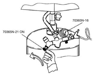
Phase 2: unscrew the valve vent-hole (part 21) and wait the discharge of the reservoir (see the hand of the manometer (part 16)). Close the valve vent-hole (part 21).
