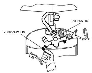
Phase 2: unscrew the valve vent-hole (part 21) and wait the discharge of the reservoir (see the hand of the manometer (part 16).
