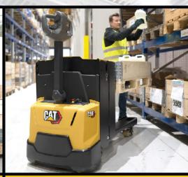
The NPP20N3E is equipped with lifting forks (730mm height) that offer an ergonomic position for loading and unloading items with minimal physical strain.
