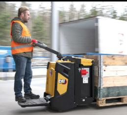
The NPP20N3R is equipped with a foldable platform for occasional use when driving over longer distances.
