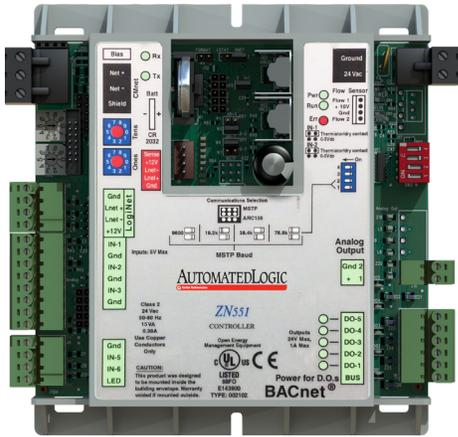
The ZN551 is a fully programmable, native BACnet Advanced Application Controller (AAC) designed for controlling a single zone in a building. The ZN551 is well suited for VAV, heat pump, unit ventilator and other packaged HVAC applications. It communicates on an EIA-485 LAN using BACnet MS/TP or BACnet over ARCNET communications and connects seamlessly to the WebCTRL® building automation system.
