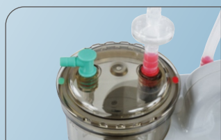
The inlet holes of VACUUM side and PATIENT side are marked by color. RED - VACUUM GREEN - PATIENT
