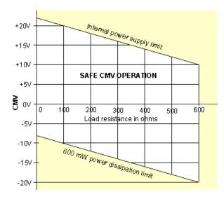
**Common mode voltage:** If a load R is grounded to a Remote Ground, the available common mode voltage CMV is limited on the positive side by the unit's internal power supply and on the negative side by the 600 mW power dissipation limit of an output transistor.
