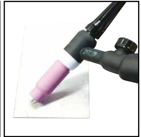
(8) Lay the outside edge of the Gas Cup on the work piece with the Tungsten Electrode 1- 2mm from the work piece.
