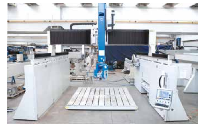
Z-axis up to 2.000 to work very high thickness pieces.
