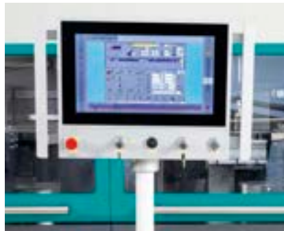
Pendulum-mounted touchscreen control panel.
