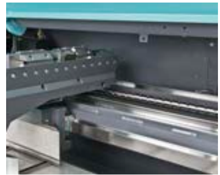
High-precision positioning of material via ballscrew driven by brushless servo motor and supported in dual linear bearings.
