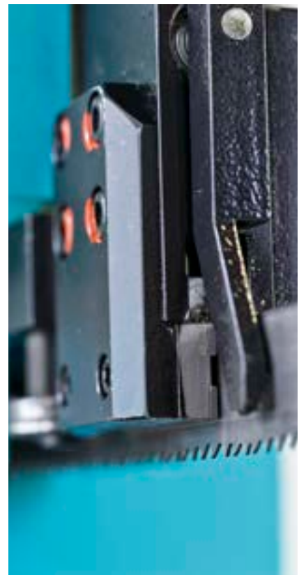
Carbide band guides for precise cuts.
