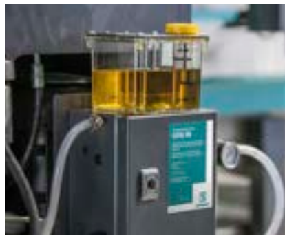
Atomiser lubrication in addition to flood coolant for virtually dry parts.
