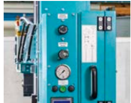
Infinitely variable hydraulic sawband feed.
