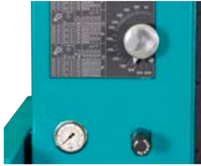
Clamping pressure reduction for thin-wall materials.
