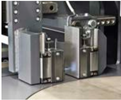
Precise material positioning via ballscrew-mounted feed gripper.
