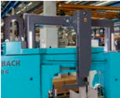
Saw bow mounted in pre-tensioned roller linear bearings.
