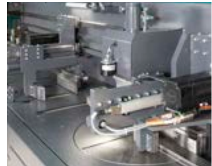
Automatic parts sorting via outfeed gripper.
