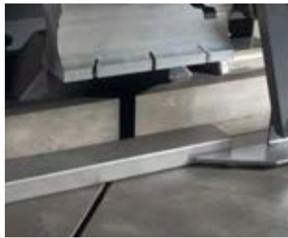
Horizontal hydraulic clamp on the outfeed holds part during the cut.
