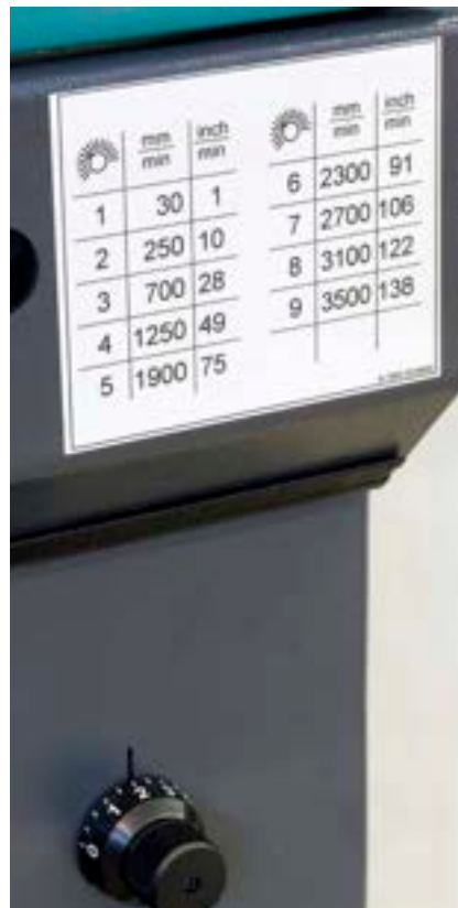
Feed regulator for infinitely variable feed setting – even during the cut.
