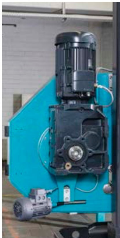
Frequency-controlled motor and gearbox mounted in a separate large-diameter roller bearing.
