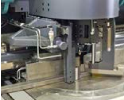
Top clamp rotates with table for optimum material clamping and shortest remnant (>15 mm).
