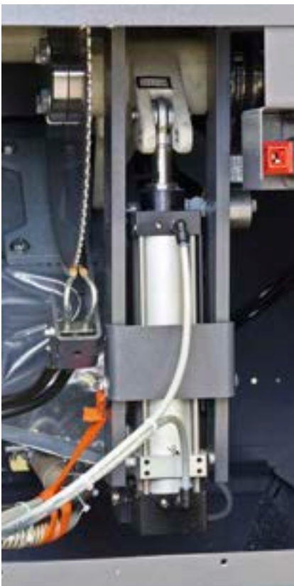
Hydro-pneumatic blade feed.
