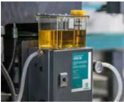
Atomiser lubrication for virtually dry parts.
