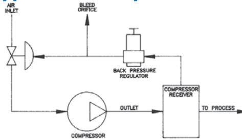
The Type 700BP is used to control the air pressure in a system supplied by a compressor. When system pressure reaches the Type 700BP set point, the unit starts relieving air pressure. This pressure is routed to an inlet valve causing it to close. Excess pressure vents through the bleed orifice and the valve opens to increase the compressor outlet pressure.
