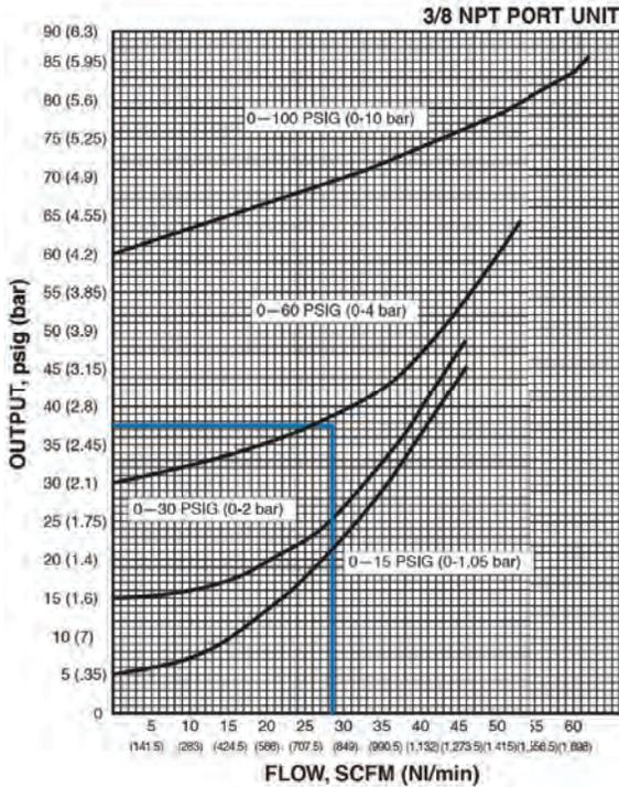
**Example:** The 0-60 psig range unit set at 30 psig will flow 28 SCFM with an 8 psig rise in pressure above the set point. All values assume relief flow is to atmosphere.
